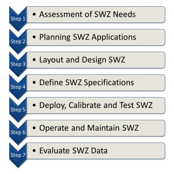
Figure 1 Process for Designing and Operating Smart Work Zones at MassDOT
