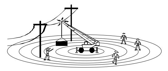
Current can flow outward through the ground in a ripple pattern from the equipment in contact with a power line.
