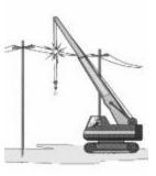
If a power line contact occurs, the operator should stay on the equipment. Don't leave unless there is an extreme emergency.
