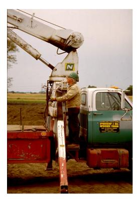
Some manufacturers offer boom truck designs which place the operator on an elevated platform, isolated from the ground.
