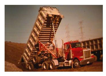
Dump trucks and other material hauling equipment often pass underneath power lines. With the truck in a raised position, the clearance around power line decreases. Careful planning as to where and how equipment is used in proximity to overhead power lines must be conducted before these trucks arrive to the job.
