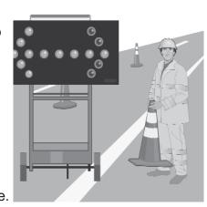
Always plan work as a "moving work zone" with proper mobile warning devices:
